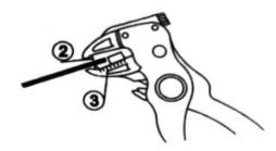
2.Clsmp prepared cable between front blades (2) for the length to be stripped.
