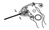
3.Press on handles: cable is locked by extrenal jaws while the insulation is lightly cut without damaging the conductor(s).For cables with particular soft or very hard sheath change hlade pressure using the adjustment(4).
