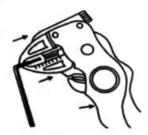
Very soft or slippery cables should be ciamped as indicated.
